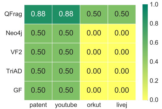
Figure 11: Fraction of queries that each system is able to successfully run for each dataset (in any configuration). All systems are able to run labeled queries, and while no other baseline is able to run any unlabeled query, QFrag successfully runs half of them. Note that Orkut and LiveJournal are unlabeled graphs so we consider only unlabeled queries, whereas in Patent and Youtube only half of the queries we consider are unlabeled.
